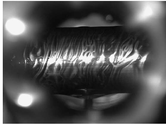
Fig. 3. Turbulent banded condensate film on condenser tube surface. Local bulk vapour concentration = 1.09 wt.% ammonia. Vapour to average outside wall temperature difference = 10.5 °C.
